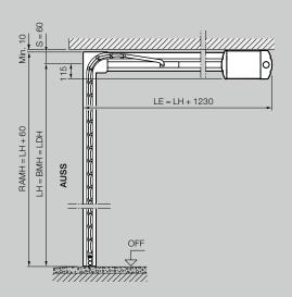
Flush-fitting in the opening with panel 95:
